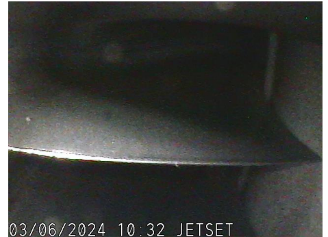
High Compressor (Impeller)
