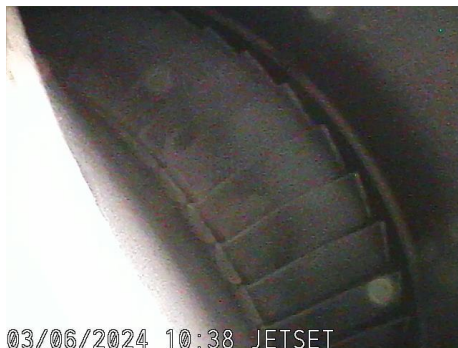
Aft Side of HT Blades
