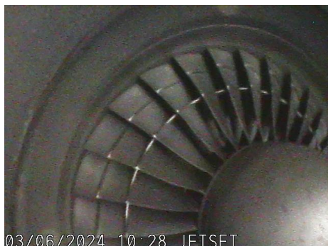
Low Compressor (Fan)
