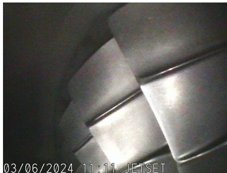
Low Compressor (Booster)
