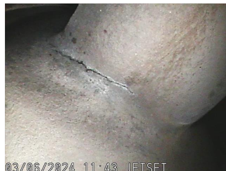
HT Airfoil Crack
