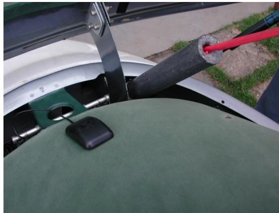
15.5 lb ballast being inserted into its proper position.
