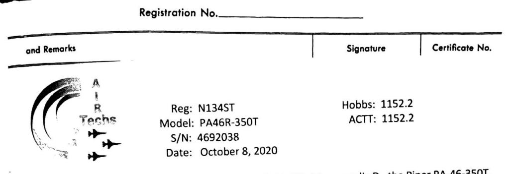
Complied with Annual inspection in accordance with 14 CER 43, appendix D, the Piper PA-46-350T, maintenance manual chapters 05-20-00 and 12-20-00. Replaced ELT battery with ME406 battery kit P/N 10-05277. ELT checked IAW FAR 91.207(d). ELT battery expires Aug 2027. Replaced Right main tire and 10-05277. ELT checked IAW FAR 91.207(d). ELT battery expires Aug 2027. Replaced Right main tire and
